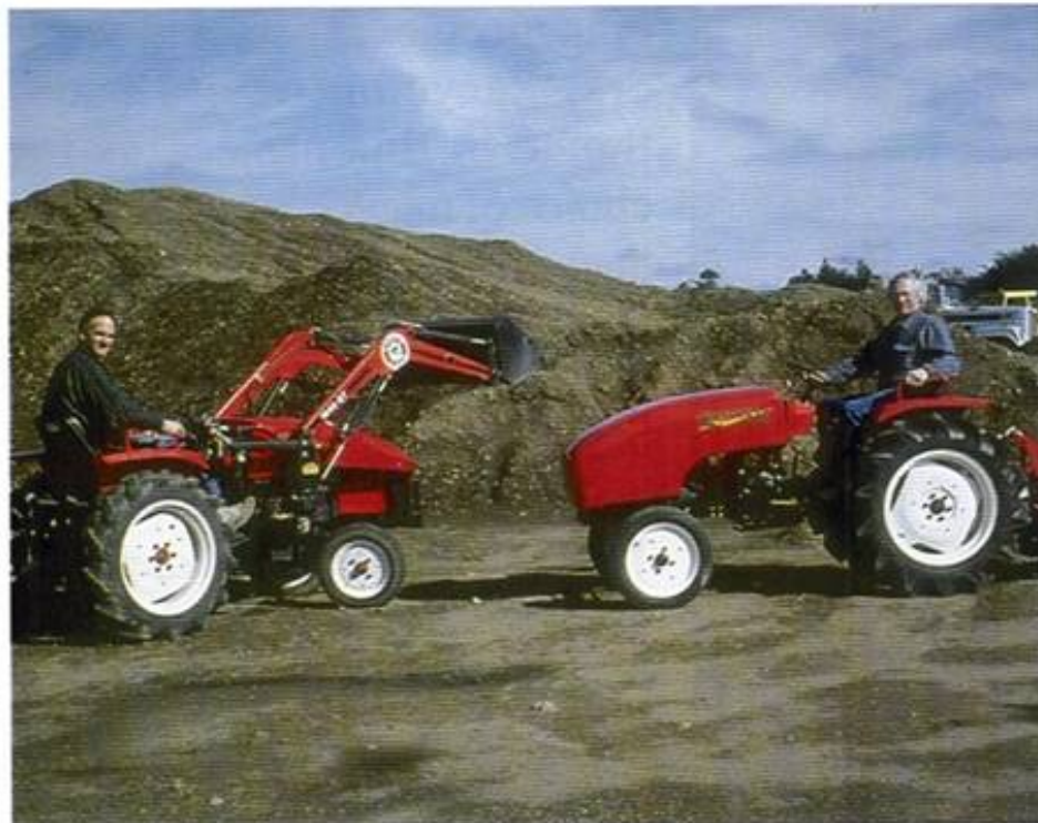
Because tractors lack emission controls and cause significant air pollution, they are ideal candidates for battery power. Tractors can also use the added weight of batteries for traction. The tractors pictured here cost $10,000 each.
