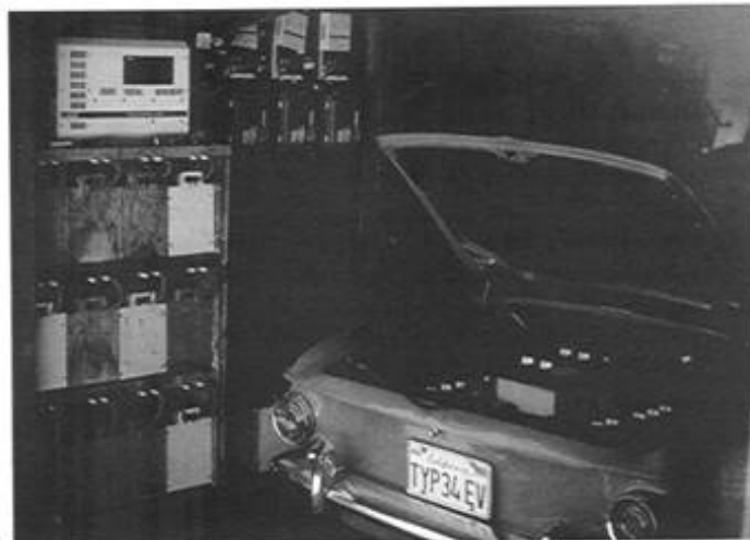
The author's Type III Karmann Ghia charging from a 3 kilowatt photovoltaic array. Batteries and a Trace 4 kW inverter are visible on the wall behind the car.
